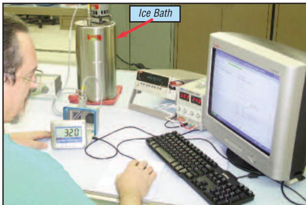
System Calibration of a Remote Digi-Stem utilizing an ice bath and USB to Computer Interface Box
