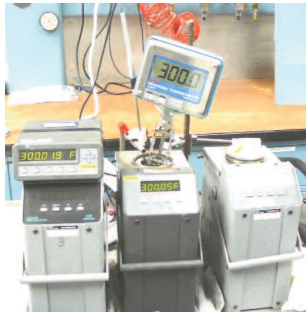
Wahl DST600 Series thermometer system being tested in the calibration lab of a major food processor, against two certified references.
