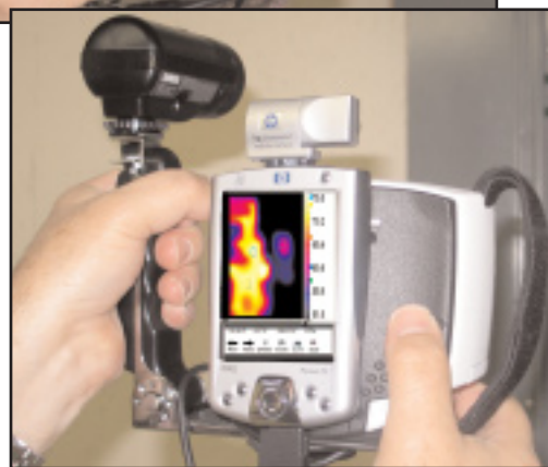
Thermal Imager Camera shown above in use mounted on the Folding Handle with Digital Camera and Light option
